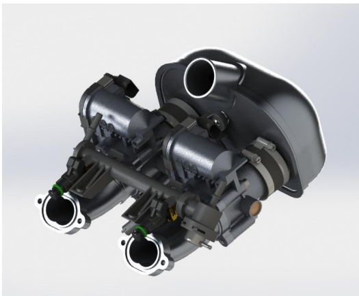
Figure 3: Electronic Throttle Body System
