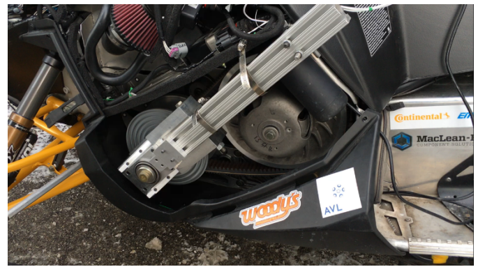
Figure 10: ECVT installed on 2016 snowmobile
