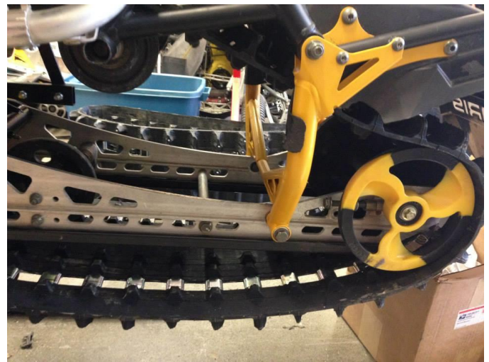
Figure 16: Offset axle and 8 inch rear idlers
