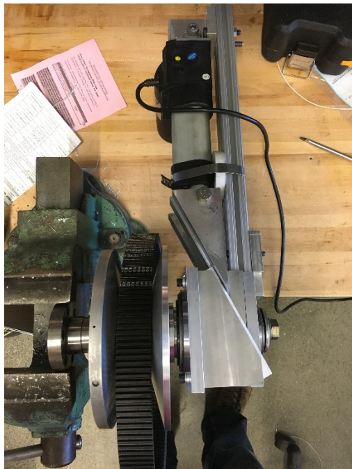
Figure 5: ECVT Mechanical System
