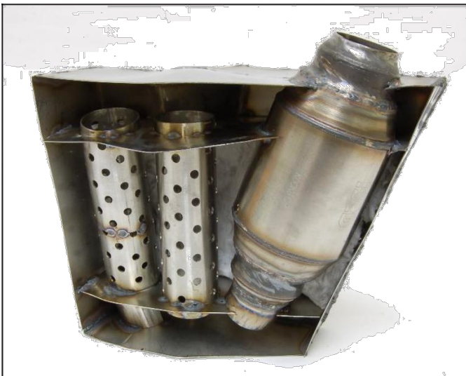
Figure 11: View of internal of baffle tubes, converter and chambers
