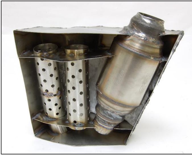
Figure 5: View of internal arrangement of baffle tubes, converter and chambers
