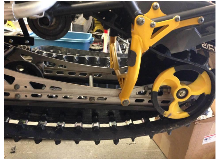
Figure 10: Offset axle and 8-inch rear idlers
