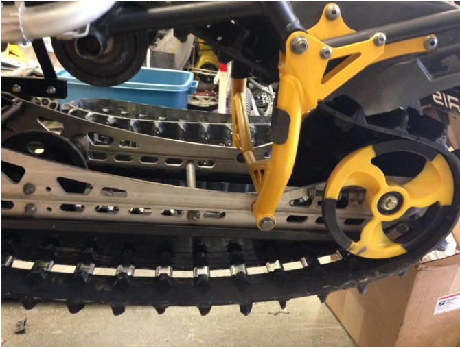
Figure 5. Offset axle and 8-inch rear idlers
