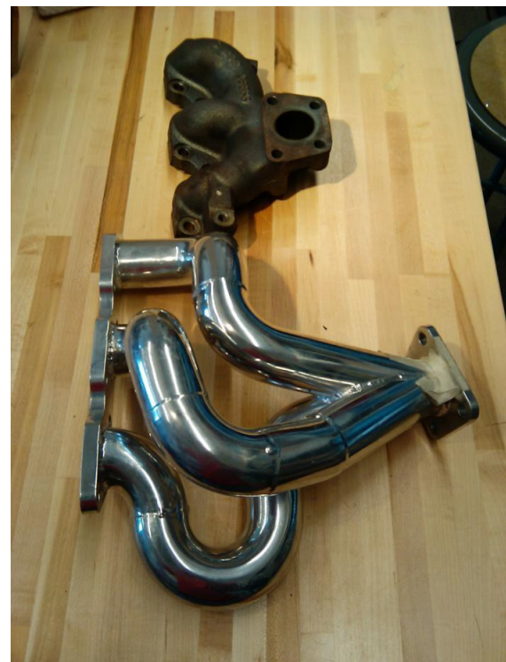
Illustration 5: Stock manifold (top) vs equal-length header (bottom)
