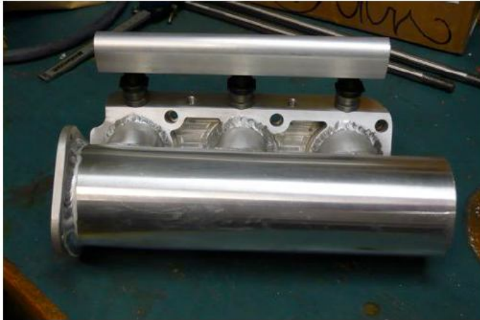
Figure 7: As-welded final air intake assembly with fuel rail mounted
