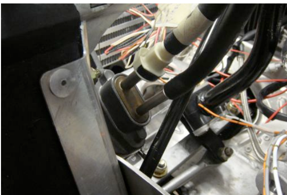
Figure 16: Flex fuel sensor mounted in location.
