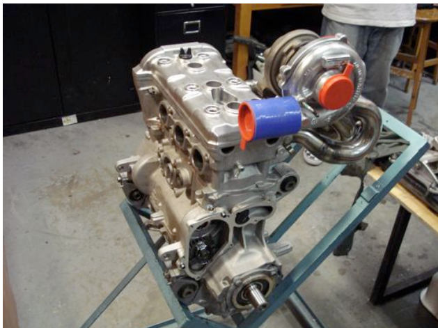
Figure 4: Turbocharger installation and custom exhaust manifold
