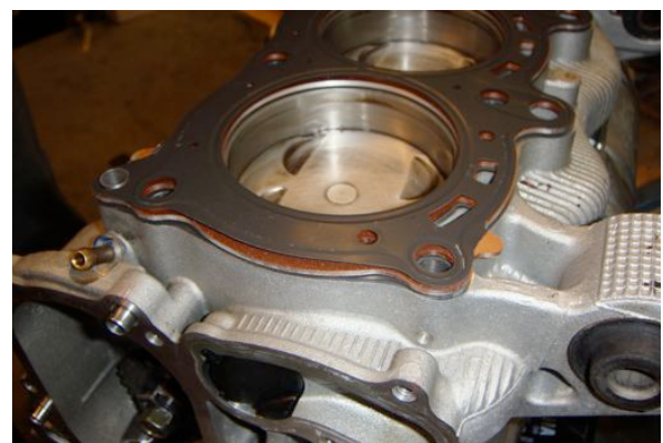
Figure 5: Installation of 2mm engine head gasket
