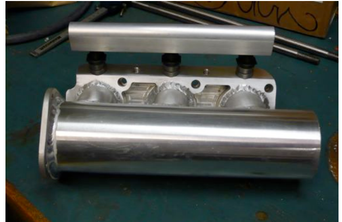
Figure 10: As-welded final air intake assembly with fuel rail mounted.
