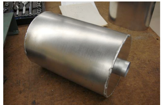
Figure 26: Exhaust silencer side-resonant element
