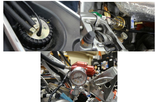
Figure 17: Fuel pump and regulator installation locations (high pressure fuel pump, low pressure fuel pump and regulator)
