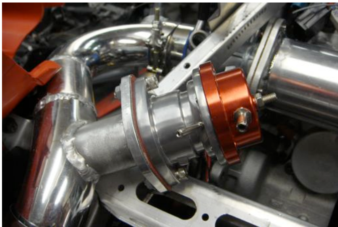
Figure 30: Blow-off valve location
