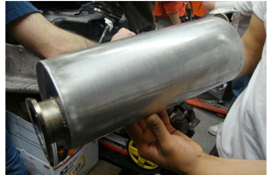
Figure 25: Exhaust silencer diffuser
