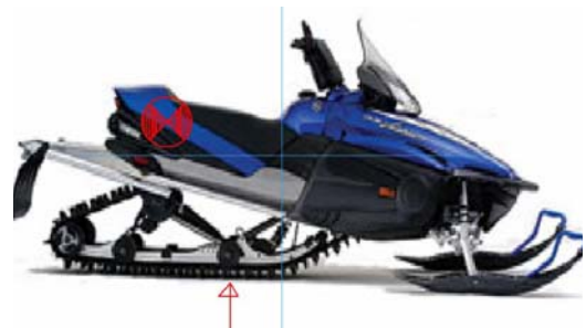
Figure 7: Contact point and center of gravity of electric sled before modifications
