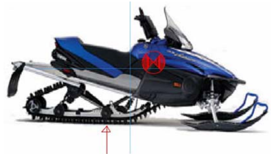
Figure 6: Contact point and center of gravity of stock sled
