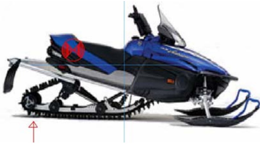
Figure 8: Contact point and center of gravity of electric sled after modifications
