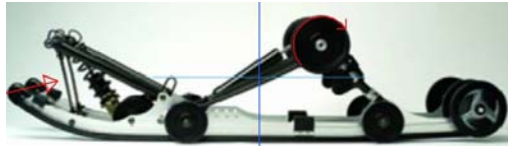
Figure 9: Effect of shortening limiting straps
