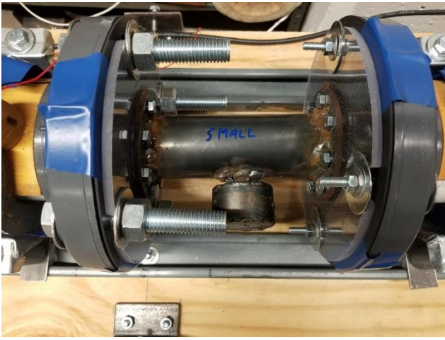
Figure 15: Picture showing a Helmholtz resonator being tested in the impedance tube.
