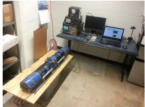
Figure 3: Impedance tube setup
