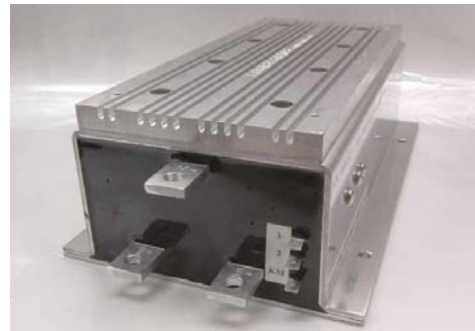
Figure 6: This is the DC brushed motor controller from Logisystems Controllers. It is manufactured in Odessa, TX and can do 137 kW continuous power. The three large connectors connect to the battery pack and motor. The three small connectors are for the variable resistor and the key switch.
