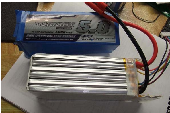
Figure 2: Turnigy 22.2 volt pack with packaging removed to show pouch cells. (Courtesy ypedal.com)
