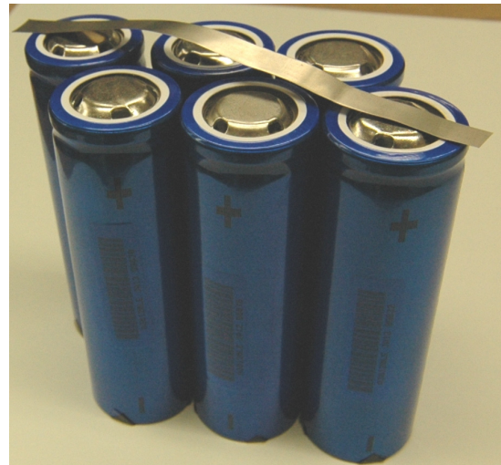
Figure 7: Each blue cylinder is a Headway 38120 10 A·h cell. Here are six of them ready to be connected with a Nickel Strip.
