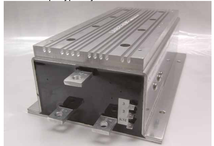
Figure 5: This is the DC brushed motor controller from Logisystems Controllers. It is manufactured in Odessa, TX and can do 137 kW continuous power. The three large connectors connect to the battery pack and motor. The three small connectors are for the variable resistor and the key switch.
