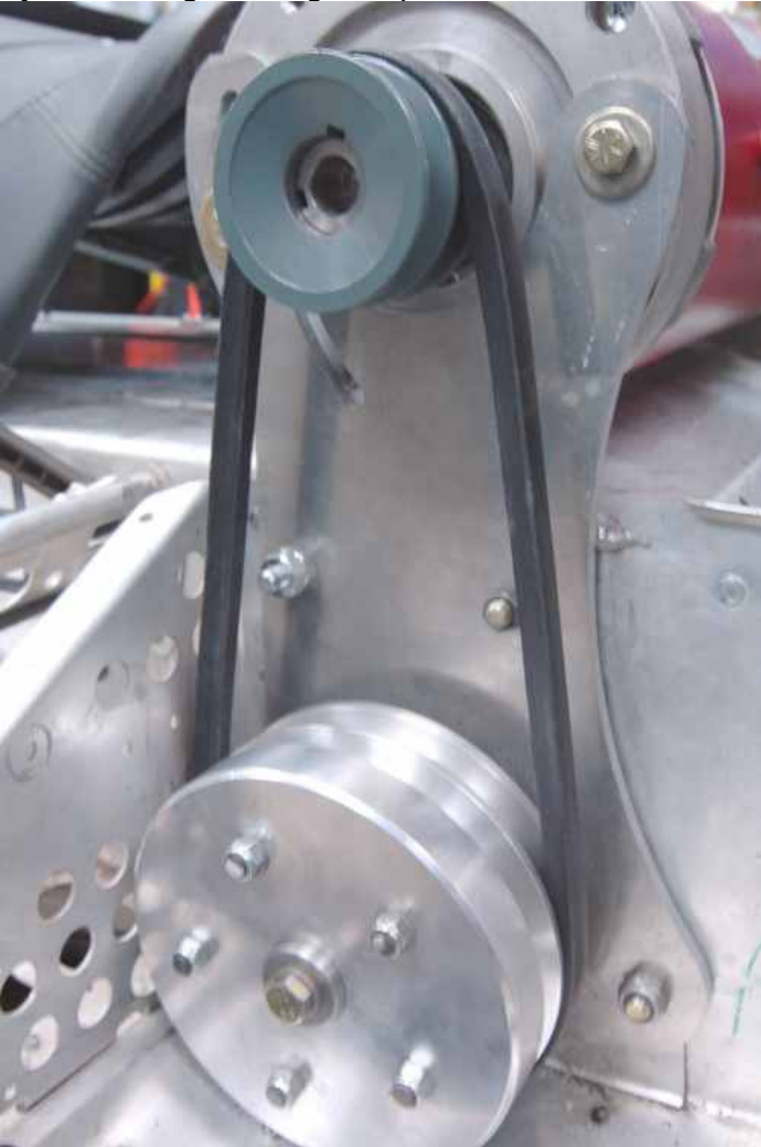
Figure 6: Two double groove pulleys are used to transmit the power from the motor to the sprocket shaft. Also pictured is the motor mount which is mounted on both sides of the tunnel.
