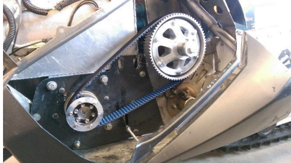
Figure 11: Belt drive with new aluminum gear.
