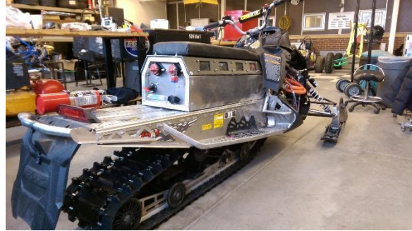
Figure 6: The battery box also serves as the seat of the snowmobile.
