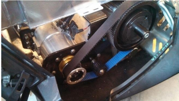
Figure 16: Belt drive from the motor to the jackshaft. Gear ratio is 3:1 (jackshaft : motor)
