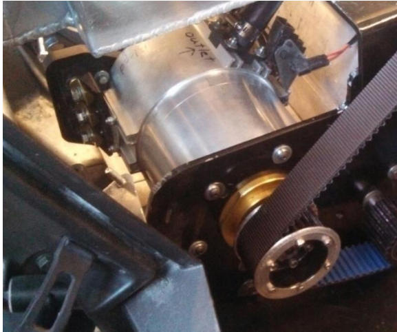
Figure 14: Liquid cooled Parker/Brammo permanent magnet AC motor.
