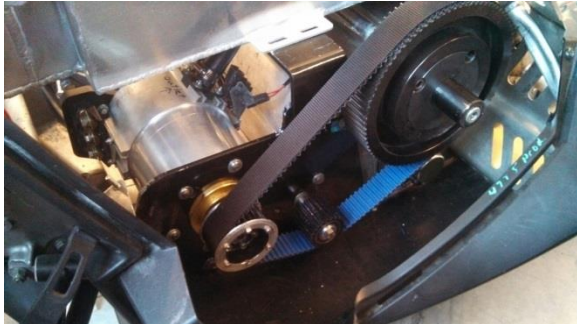
Figure 13: Belt drive from the motor to the jackshaft. Gear ratio is 3:1 (jackshaft : motor)
