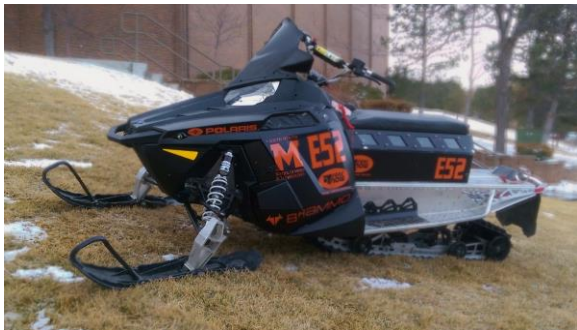
Figure 15: The seat is comfortable and provides an ergonomically correct riding position. ProTaper handle bars offer both stand up and sit down comfort.
