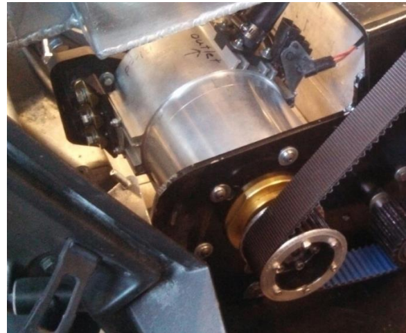
Figure 10: Liquid cooled Parker/Brammo permanent magnet AC motor.
