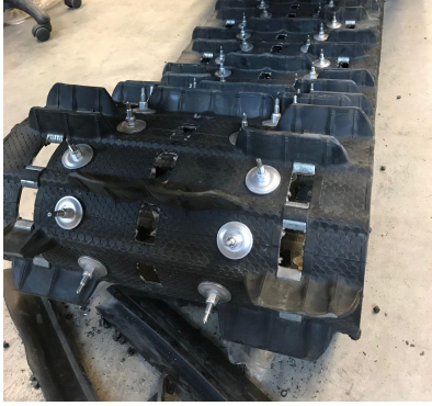
Figure 7: Track with Wood's Traction studs
