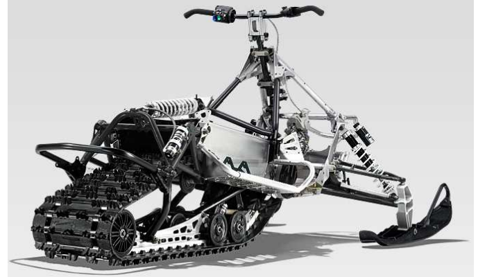
Figure 14: 2014 Polaris Pro-Ride chassis.
