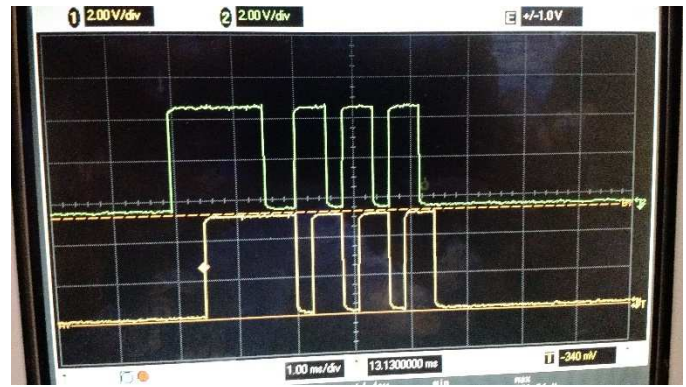
Figure 11: DCCDI 5V trigger signal from external module.
