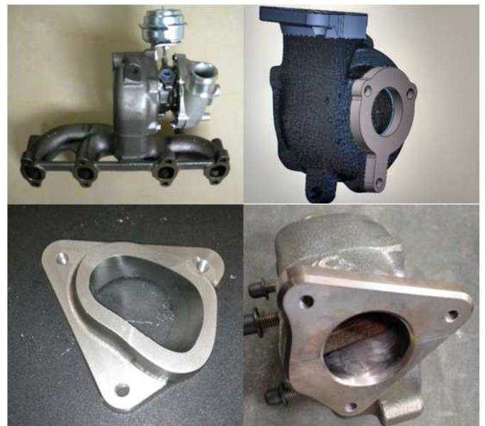
Figure 9: 3D scan, CAD design, machined flange, and assembled turbine housing.
