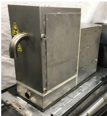
Figure 6. Blackthorn Diesel Particulate Filter
