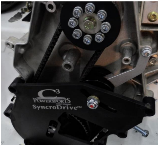
Figure 4. C3 belt drive system
