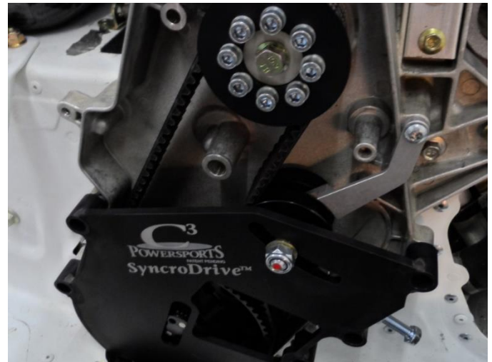
Figure 3: C3 SyncroDrive Belt Drive
