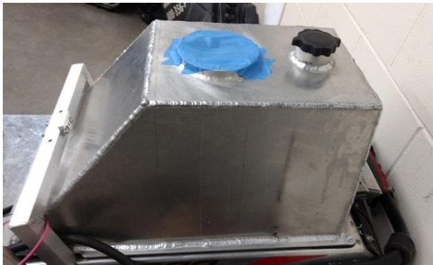
Figure 13: Custom Fuel Tank
