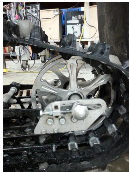
Figure 4: Ten inch wheels with 136 inch track
