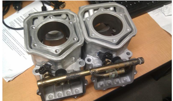
Figure 5 Photo of UW Platteville's Supplemental Injectors
