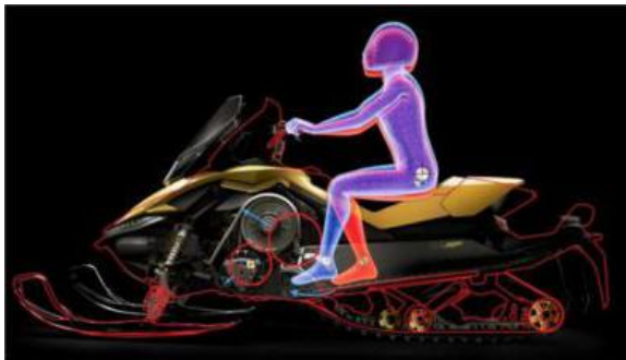
Figure 4: Red outline shows the riding position and layout of a previous Rev chassis. The blue outline shows the current Rev-XP chassis [15].
