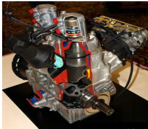
Figure 2: Cross section of a 2011 800R E-TEC, similar to the 600 E-TEC. [15]
