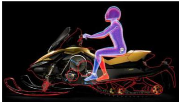
Figure 3: Red outline shows the riding position and layout of a Ski-Doo Rev. The blue outline shows the Rev-XP [16].
