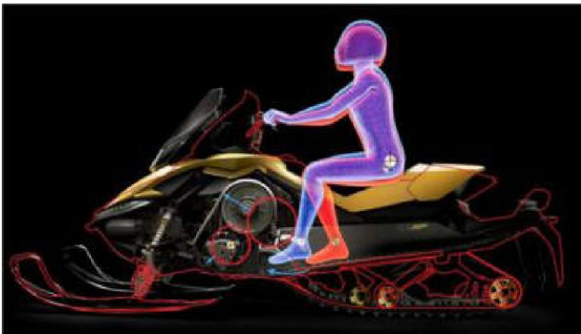
Figure 4: Rider forward positioning of 2008 Rev-XP (outlined in blue) versus 2007 Rev (outlined in red) [12].
