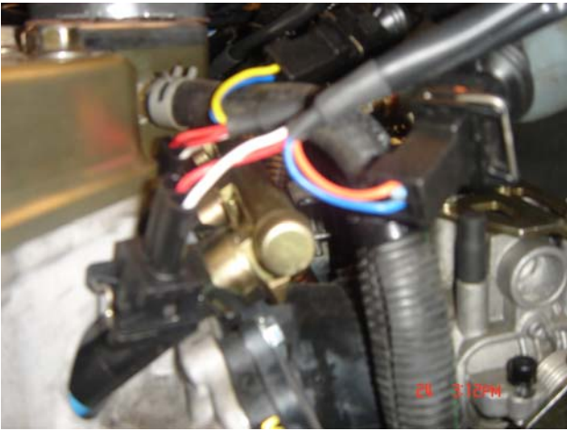
Figure 9: Full Flex kit connected to injectors
