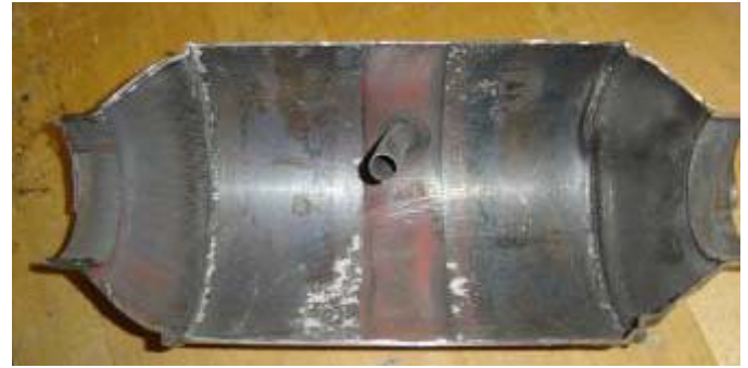
Figure 22: Cut-Away Section of Catalyst Housing
