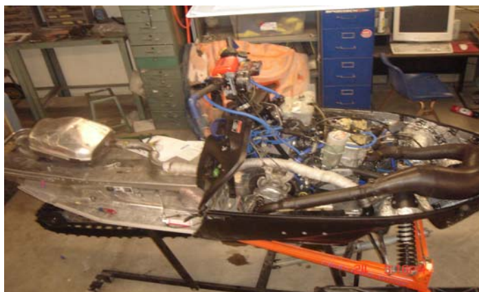
Figure 13: Pro-X with Modified Exhaust System
