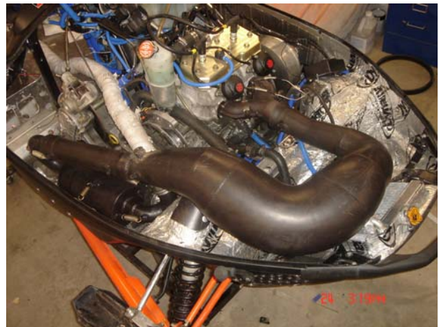
Figure 15: Custom AAEN Pipe and Expansion Chamber
