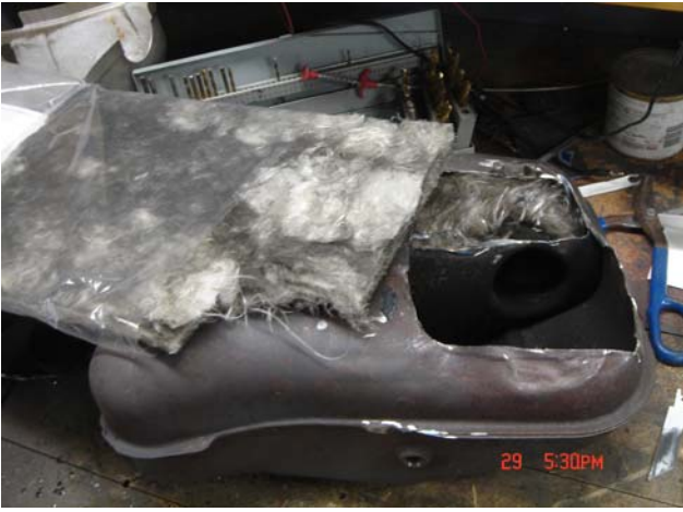
Figure 5: Modified Rotax 600cc Silencer
