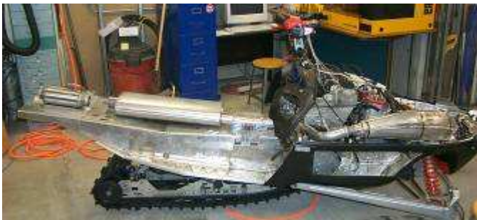
Figure 10: Pro-X with Modified Exhaust System
