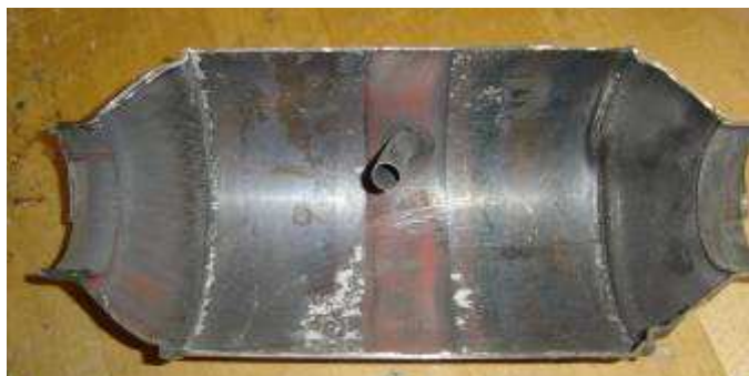
Figure 20: Cut-Away Section of Catalyst Housing
