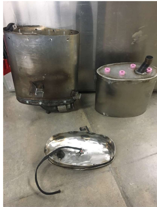
Figure 8. Bottom view of DPF with inside chamber.
