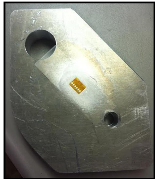
Figure 2.3: Rosette Strain Gauge on Relocation
