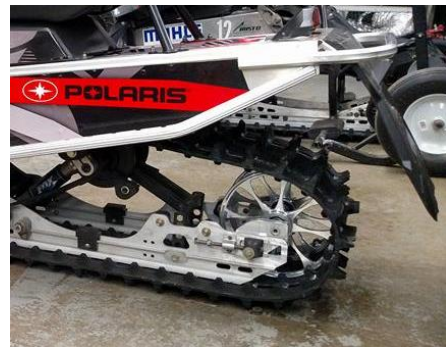
Figure 3: Big Wheel Kit on Polaris Indy
