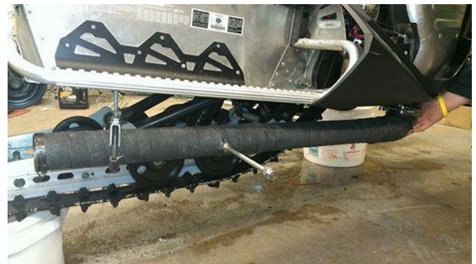
Figure 10: Emissions Test Pipe
