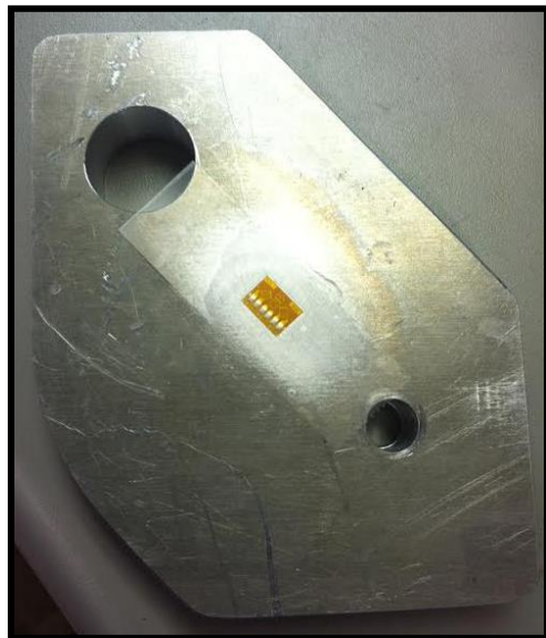
Figure 5: Rosette Strain Gauges on Mock Skid
