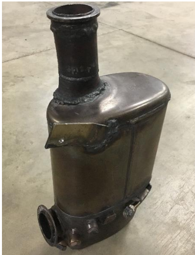
Figure 10. Volkswagen Wall Flow DOC/DPF system
