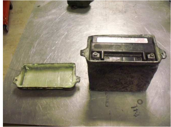
Figure 06: Sealed battery Box
