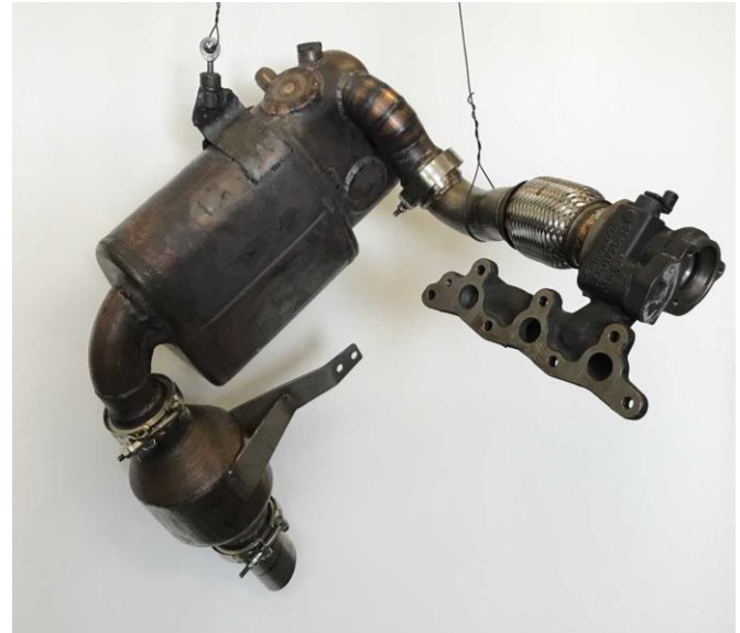
Figure 3. Exhaust and Aftertreatment System
