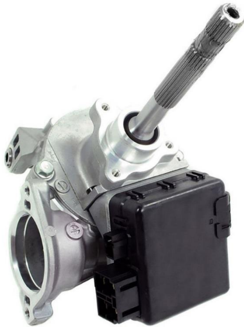
Figure 9: Saturn Vue electronic steering assist motor assembly
