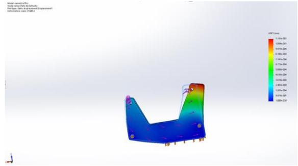
Figure 16. FEA Displacement Results of Left Hand Side Motor Mount Plate Due to Motor Torque
