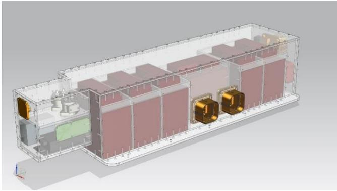
Figure 2. MTU Zero Emission Battery Containment Unit
