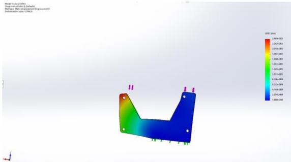
Figure 14. FEA Displacement Results of Left Hand Side Motor Mount Plate Due to Motor Weight
