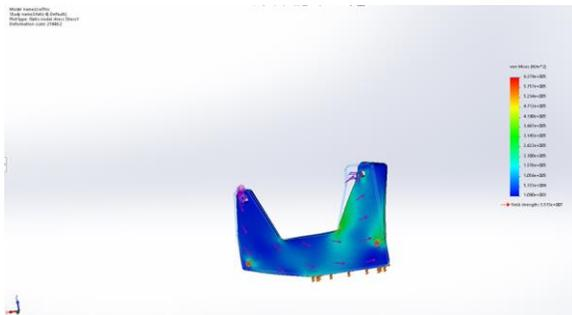
Figure 15. FEA Stress Results of Left Hand Side Motor Mount Plate Due to Motor Torque
