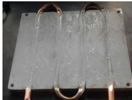
Figure 8. Chill Plate with Thermal Paste
