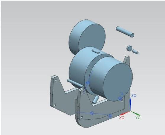
Figure 11. CAD Model Assembly of the Motor and Motor Mount Plate Showing all Geometry
