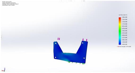
Figure 13. FEA Stress Results of Left Hand Side Motor Mount Plate Due to Motor Weight
