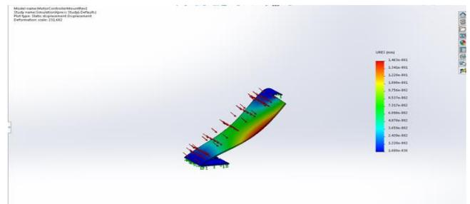
Figure 5. Deflection FEA Results on the Motor Controller Mount
