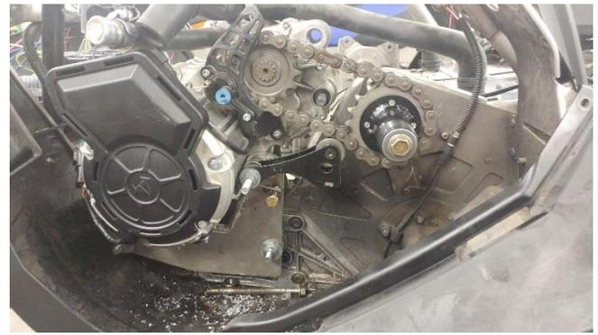
Figure 12. Physical Assembly of Fabricated Drivetrain System Including the Motor, Motor Mount, Chain Drive, and Tensioner
