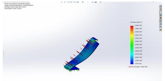
Figure 6. Stress FEA results on the Motor Controller Mount
