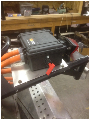
Figure 9. Master Switch Relocation
