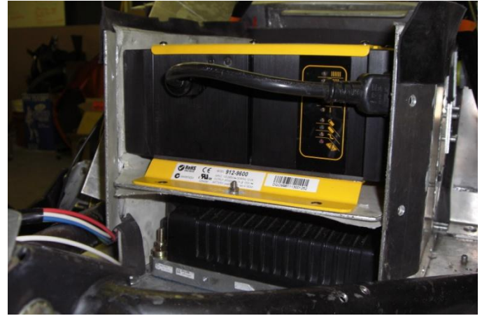
Figure 1. Charger and controller mounting location.
