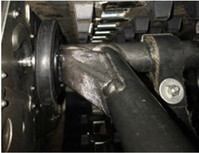
Figure 8: Modified Front Torque Arm with Circular Roller
