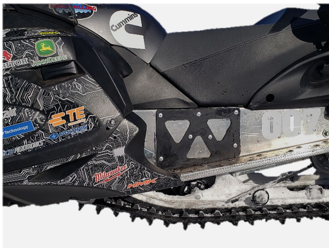
Figure 13: Vibration Reduction Plates Mounted to Tunnel
