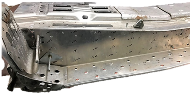
Figure 9: Yamaha Venture Tunnel with Impact Testing Locations
