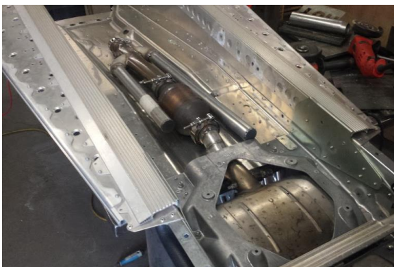
Figure 22. Modified Exhaust with Quarter Wave Resonator
