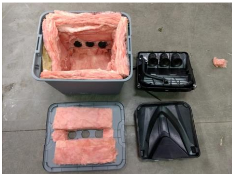
Figure 2. Overkill Airbox Compared to OEM Airbox
