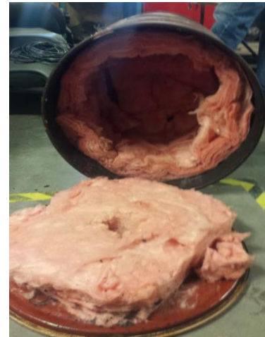
Figure 3. Overkill Muffler Internals
