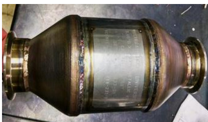
Figure 13. 2018 Three-Way Metallic Catalytic Converter
