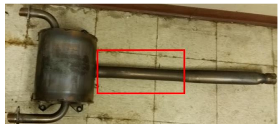
Figure 14. Proposed Catalyst Location
