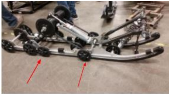
Figure 25. Removed Bogey Wheel Sets
