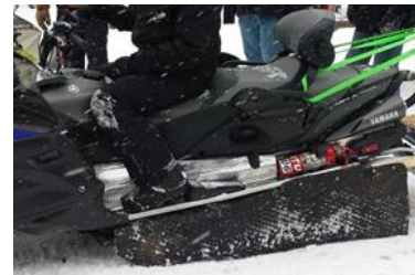
Figure 27. Prototype Track Skirt Made of Thick Rubber
