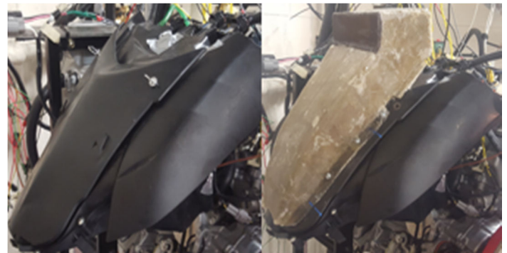
Figure 17: Original air box lid vs prototype lid
