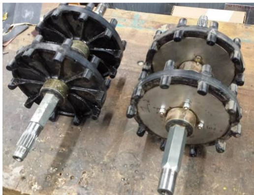
Figure 20: Stock drivers (left) and completed custom isolated drivers (right)
