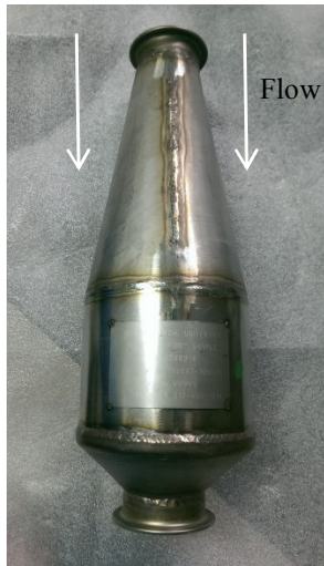
Figure 8: The catalytic converter that will be used in the MTU exhaust system that will reduce the levels of UHC, NO x and CO
