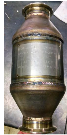
Figure 8: Three way catalyst that will be used in the MTU exhaust that will reduce the levels of unburned hydrocarbons, \text{NO}_x CO, and \text{CO}_2
