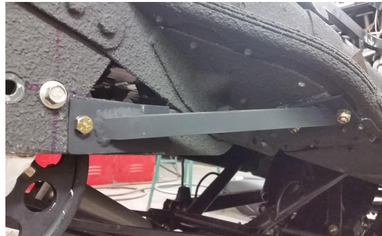
Figure 12: Support bracket created to provide lateral support to the skid brackets
