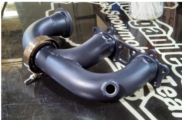
Figure 8: Completed header with ceramic coating
