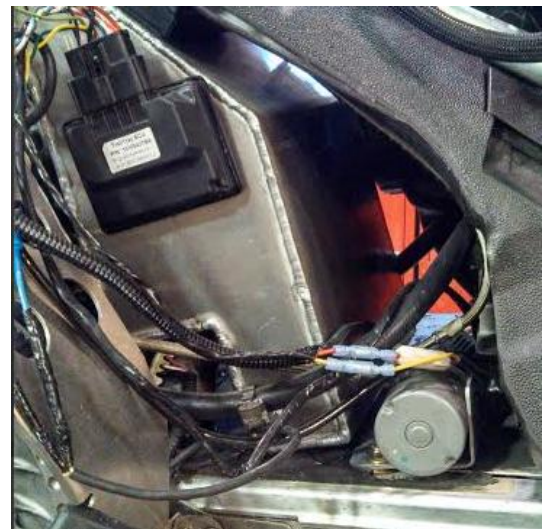
Figure 18: Hayes HCU and HECU mounting locations.
