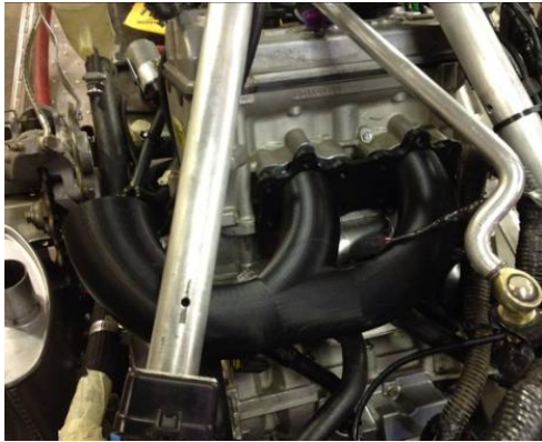
Figure 6: Test fit of 3D printed model of header
