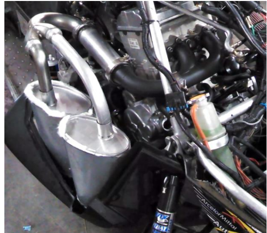
Figure 9: Final stages of exhaust fabrication
