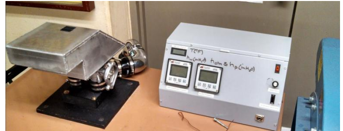
Figure 5: Flow Bench Testing
