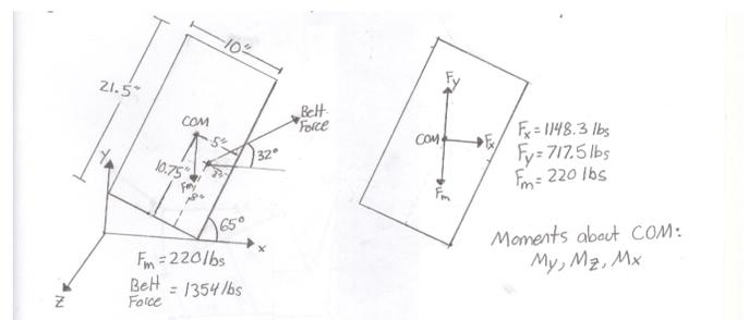
Figure 6: Forces on center of mass due to belt tension.
