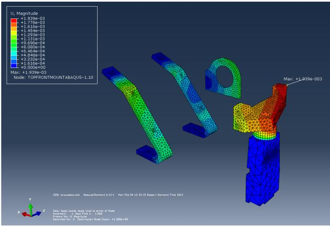
**Figure 10: Displacement Contour Plot of Mounting System.**
