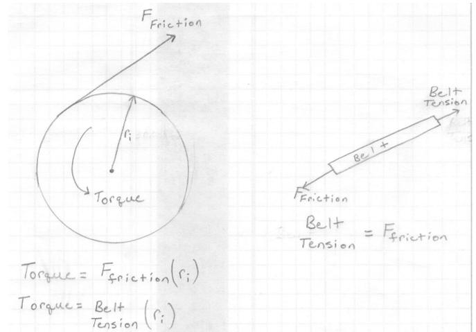
Figure 5: Free body diagram to determine belt force.
