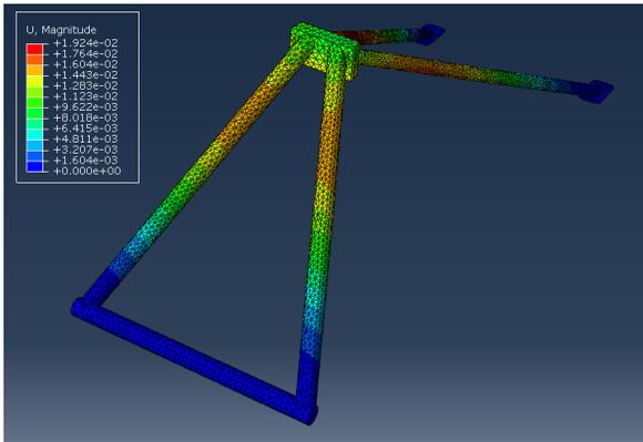
**Figure 14: Displacements in New A-frame Design.**
