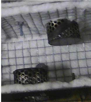
**Figure 22: Inside view of exhaust with packing and perforated tube.**
