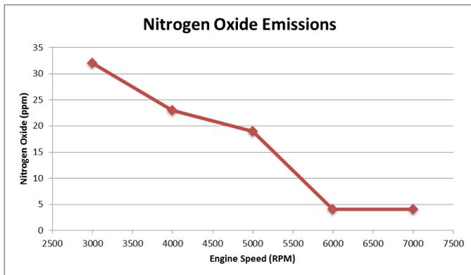
Figure 25: NO<sub>x</sub> levels at varying RPMs.
