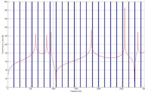
**Figure 19: Matlab results for single chamber muffler.**
