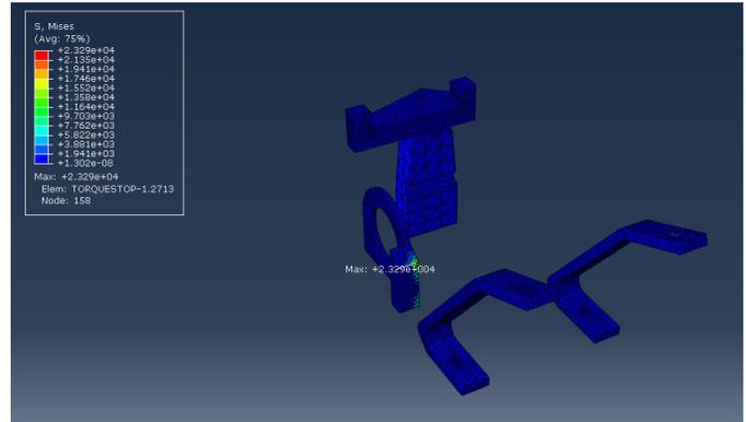
**Figure 8: Von Mises contour plot of entire system.**
