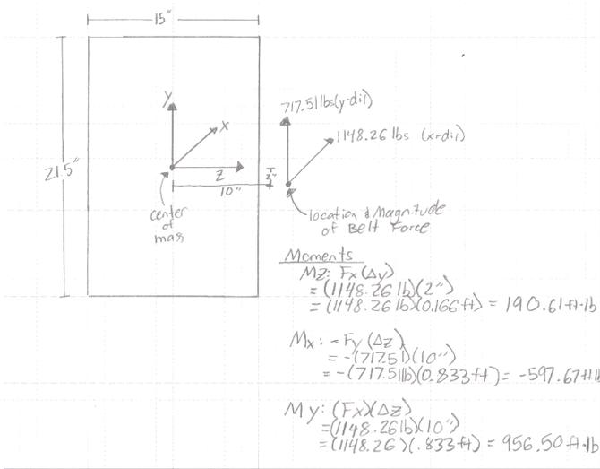
**Figure 7: Front View of Engine and Moments on Center of Mass Due to Belt Tension.**
