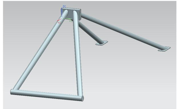
**Figure 12: CAD Drawing of new A-frame design.**
