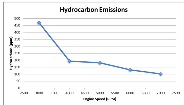
**Figure 23: Hydrocarbon levels at varying rpms**
