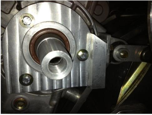
Figure 4: Torque stop after machining.
