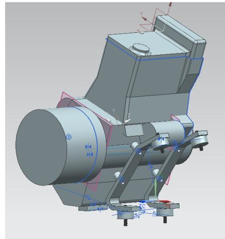
*Figure 2: CAD model of rear engine mounting system*
