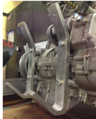
*Figure 1: Rear engine mounts on engine*
