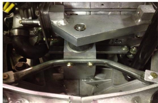
*Figure 3: Front engine mount with bracing*
