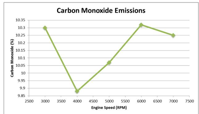
**Figure 24: Carbon monoxide levels at different RPM levels.**
