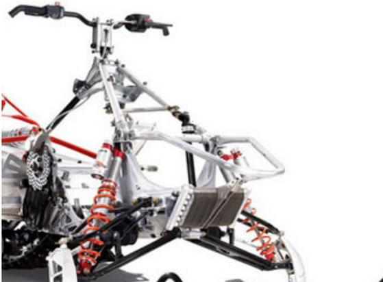
**Figure 11: Stock over structure and steering system**
