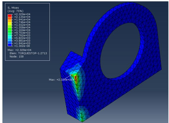
**Figure 9: Von Mises Contour Plot of Torque Stop Plate.**
