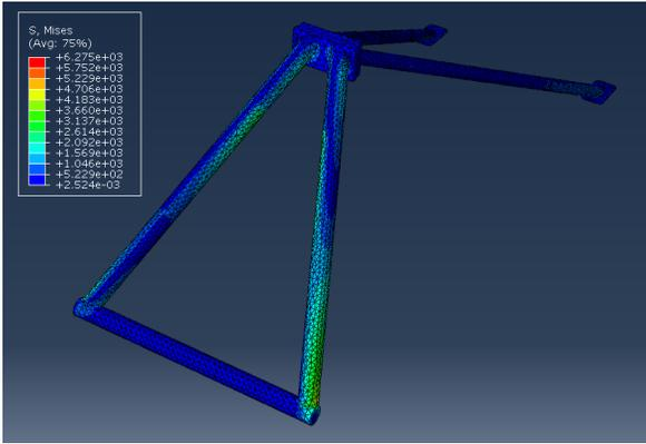
**Figure 13: Von Mises Stresses in New Over Structure Design.**
