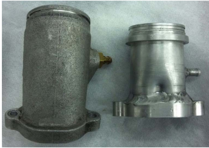
Figure 2: Stock intake runners (left) and MTU designed intake runners (right)
