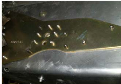
Figure 14: Tunnel Reinforcement Plate
