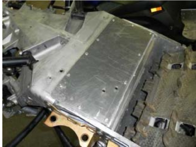
Figure 9: Bulkhead Reinforcement Plate
