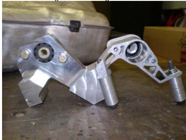
Figure 7: Front stator side engine mount (left) next to stock mount (right)
