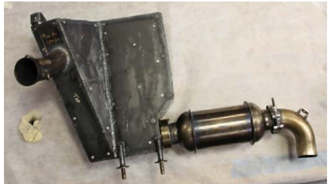
Figure 6: Backside of MTU designed exhaust
