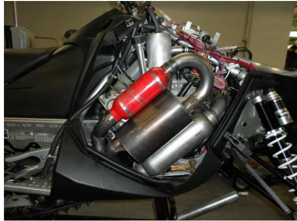
Figure 16: Exhaust Mounted in Chassis
