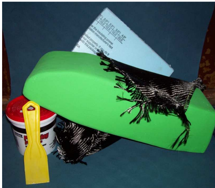
Figure 12: The Finished Airbox Mold with raw 3K 2x2 twill Carbon Fiber and some needed Supplies
