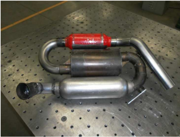
Figure 15: Finished Exhaust System
