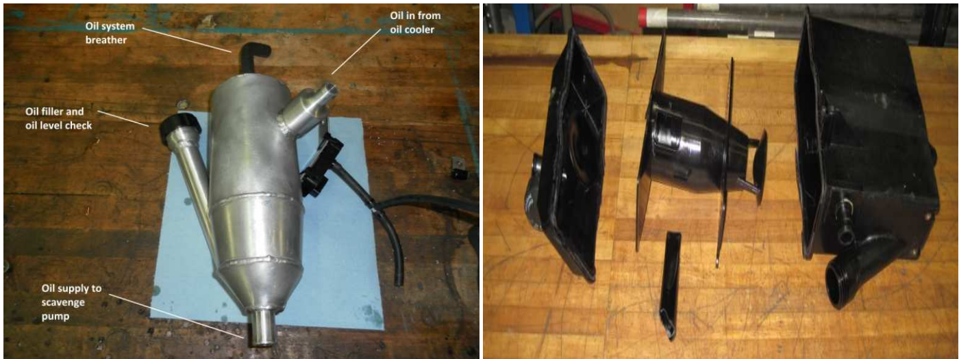
Figure 18: MTU Designed Oil Bottle and Stock Oil Bottle Internals
