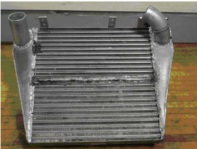
Figure 2.1: This picture displays the 2009 MTU designed and fabricated air to air intercooler.
