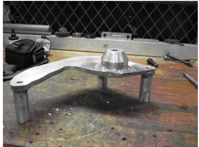
Figure 2.3: This picture depicts the 3/8" thick aluminum engine mount plate made to accommodate the stator implementation.
