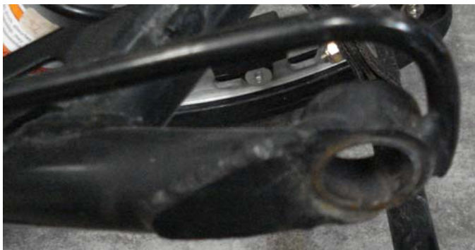
Figure 4.0: This picture displays the modifications made to the front torque arm of the SC-5 rear suspension.
