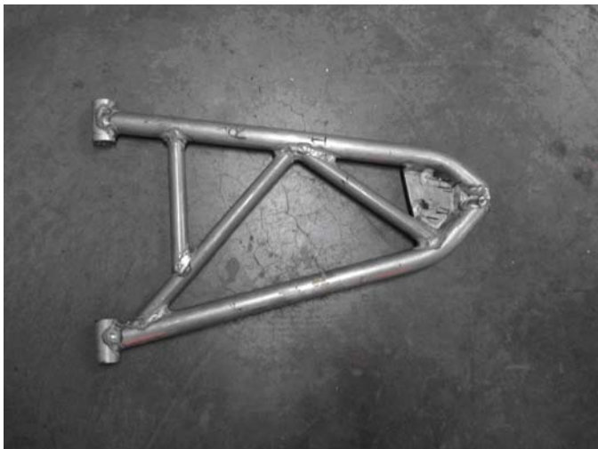
Figure 5.2: This picture shows an aluminum lower A-arm.
