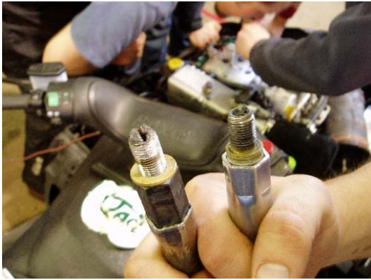
Figure 6. 2004 Pre-Combustion Chamber Failure
