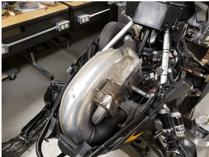
Figure 1. Modified exhaust system with no exhaust wrap.
