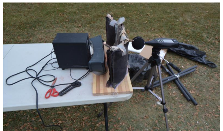
Figure 9: Sound testing rig in use, with Brüel and Kjær 2270 Sound Level Meter
