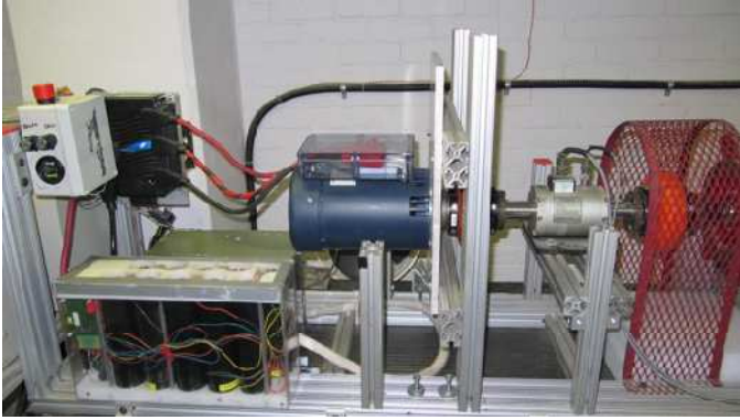
Figure 1: Electric Dynamometer Setup
