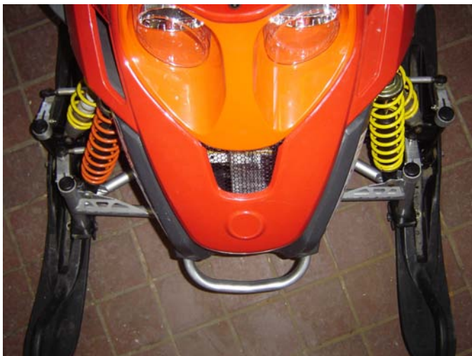
Illustration 8: 2006 suspension superimposed onto the 2007 suspension
