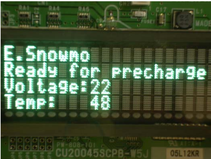
Illustration 10: Electric Snowmobile high brightness VFD
