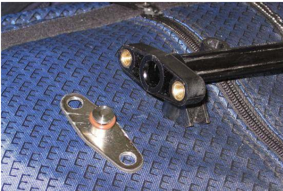
Figure 6: Machined plug for the stock fuel rail
