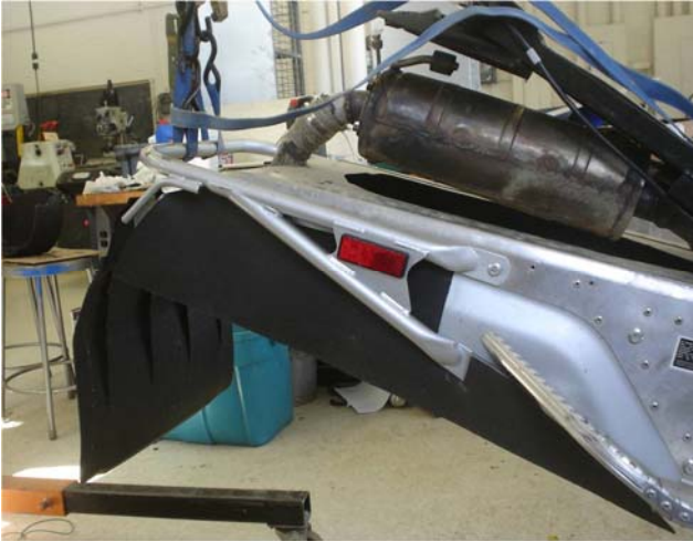
Figure 18: Side skirts attached to the snowmobile's tunnel
