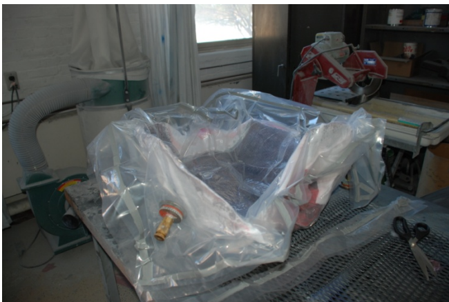
Figure 9: Finished vacuum bagged fiberglass side panel
