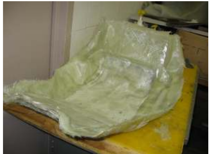
Figure 16. Lower mold half, laid up with fiber
