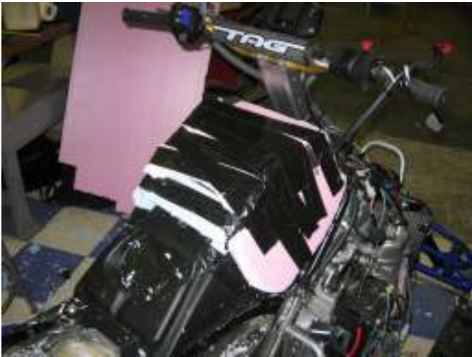
Figure 13. Stock tank with added foam
