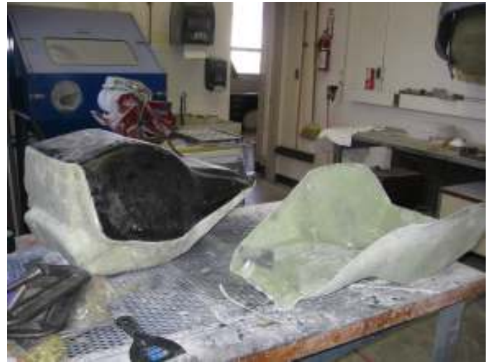
Figure 15. Finished plug with mold halves
