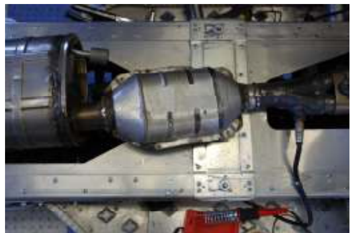
Figure 10. Catalytic Converter welded before muffler
