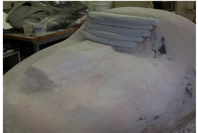
Figure 2: Windshield plug modification
