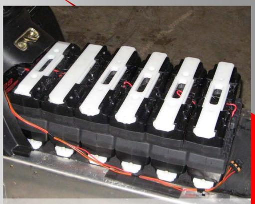
7 strings x 2.8 A-hr = 19.6 A-hr 84 cells x 4 V/cell = 336  $V_{nominal}$
